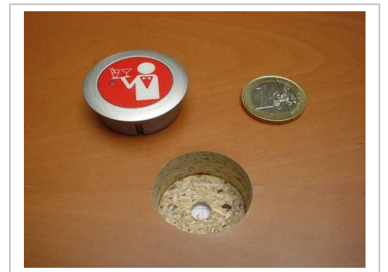
Mounting hole: 30mmØ x 15mm depth plus drainage
